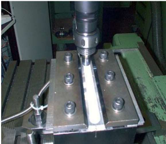
Fig: 1.1.1: Friction stir welding process
